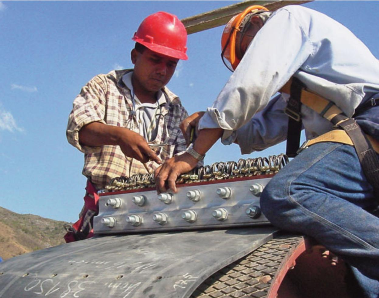
Splicing of steel-reinforced belt
