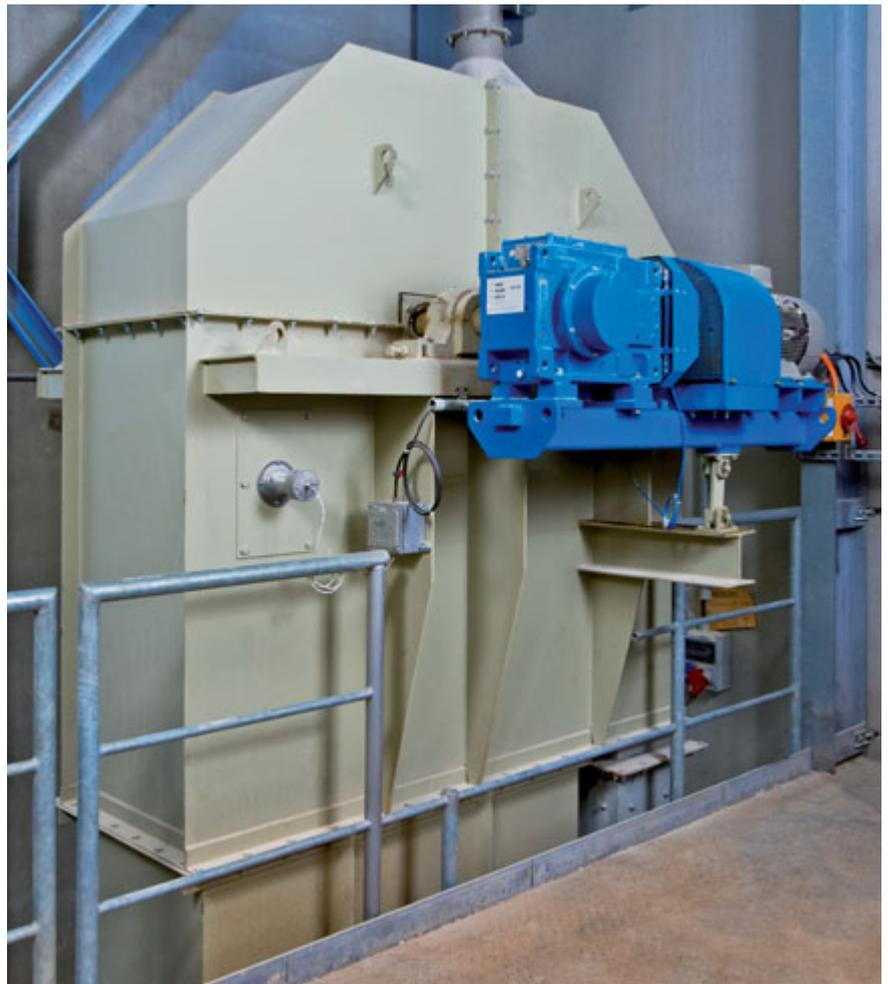
Bucket elevator head with single drive
