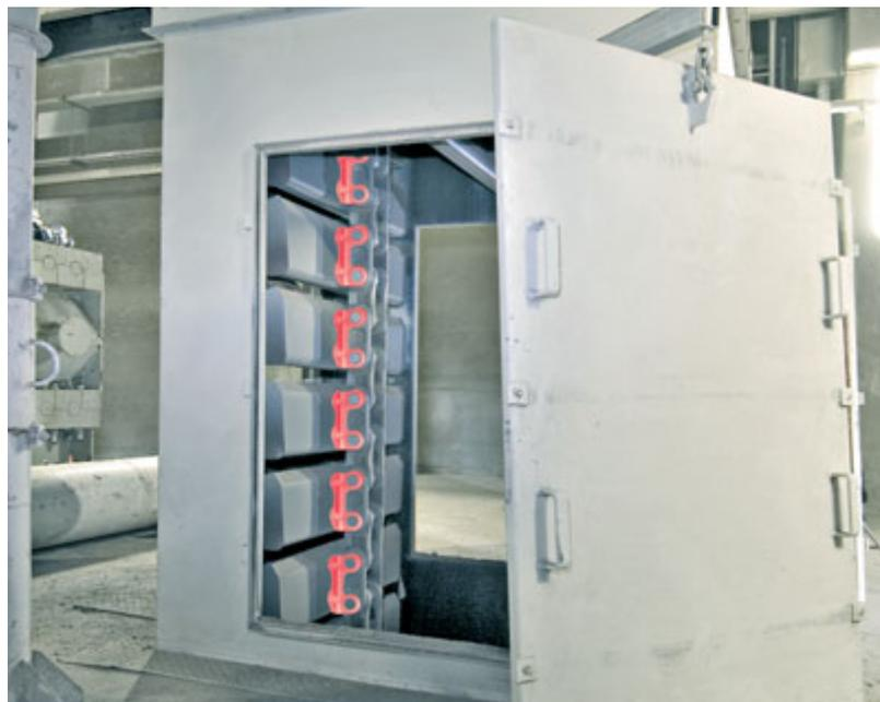
Assembly casing with hinge-supported door for easy maintenance
