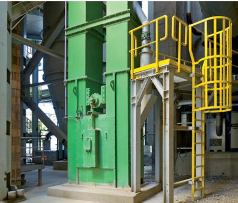
Elevator boot with parallel tensioning device
