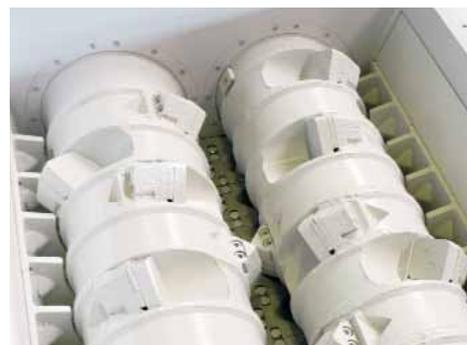
Rotors of the double-shaft pre-shredder
