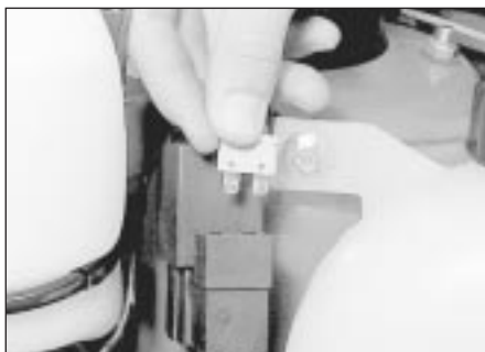
3.7b Removing the headlamp washer fuse
