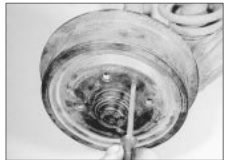
9.3a Removing a brake drum securing screw
