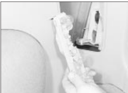
11.16b Rear lamp cluster bulbs and holder
