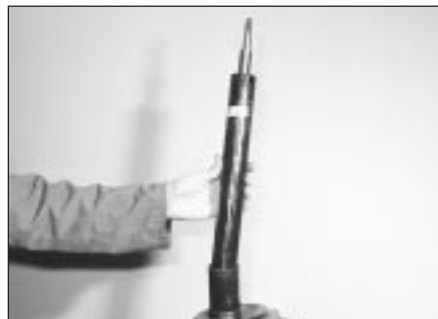
4.7 Removing the shock absorber cartridge
