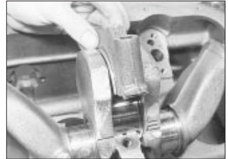
20.14 Fitting the centre main bearing cap
