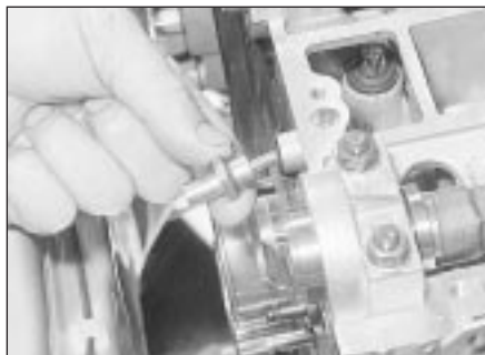
11.18b . . . and the belt cover mounting stud
