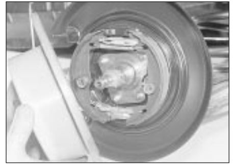
8.5 Removing the rear disc
