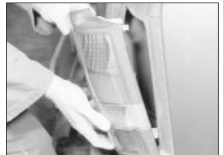
11.17b Removing a rear lamp lens
