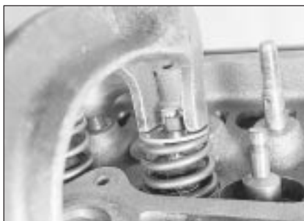
9.20 Compress the spring and fit the collets
