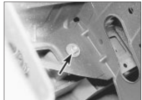
8.3 Front trim panel securing nut (arrowed)
