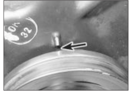
7.7 Ignition timing marks (arrowed) in alignment
