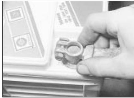
4.2 Disconnect the battery negative terminal first
