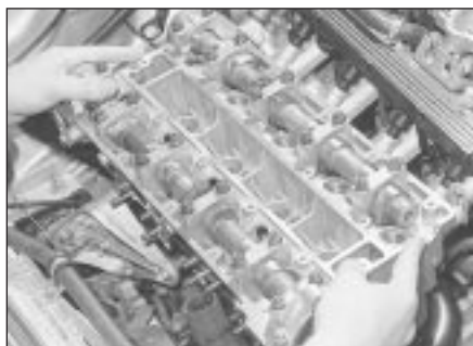
11.20 Lifting off the cylinder head
