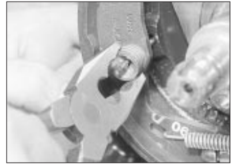
20.3a Removing a steady washer . . .
