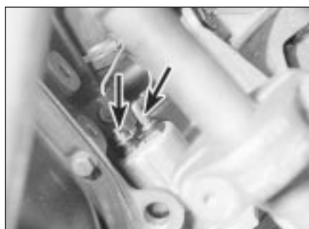
13.2 Oil pressure sender wires (arrowed)
