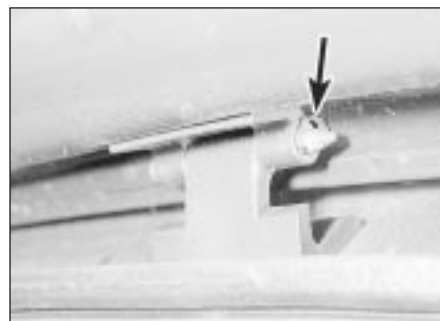
20.4 Tailgate hinge showing circlip (arrowed)
