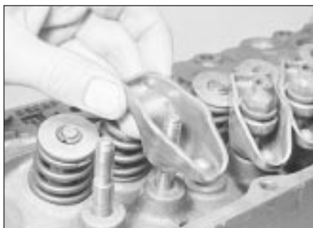
9.24a Fitting a rocker arm . . .
