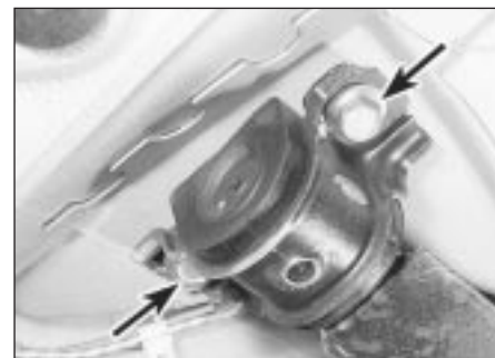
5.4 Control arm clamp bolts (arrowed)
