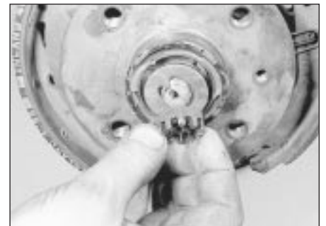
10.6b . . . the washer and the castellated nut
