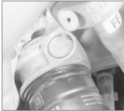
16.2 Circlip securing oil cooler thermostatic valve
