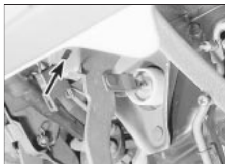
17.1 Stop-lamp switch 'keyhole' mounting (arrowed)
