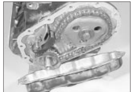
14.21 Refitting the timing cover
