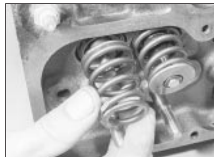
9.18a Fit the valve spring . . .
