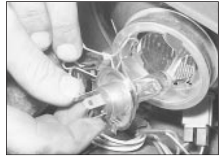
11.3 Removing a headlamp bulb
