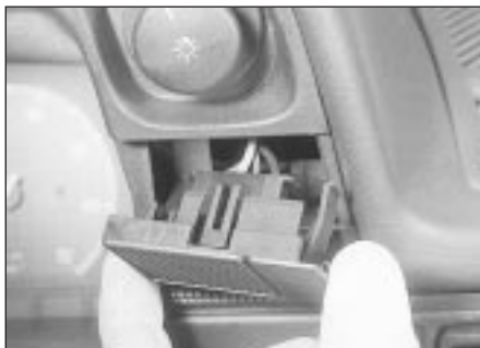
4.5 Removing a foglamp switch
