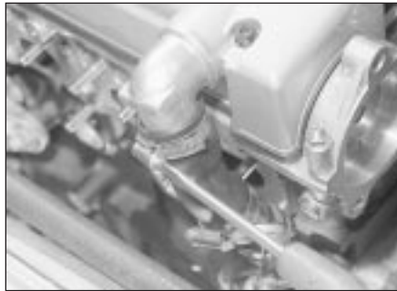
11.15 Disconnecting the large breather hose
