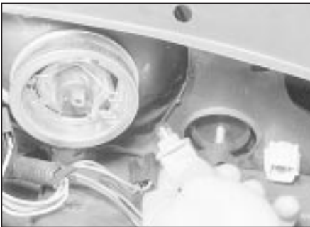
11.7 Removing a sidelamp bulb and holder
