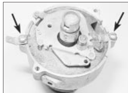
7.7 Undo the baseplate retaining screws (arrowed)
