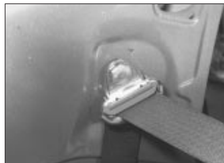
37.7b Rear seat belt upper mounting
