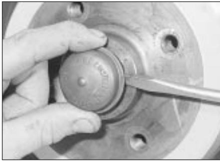
8.3 Levering off the grease cap
