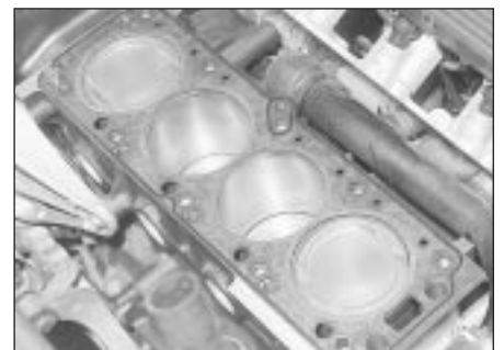
11.22 New head gasket in position
