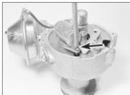
7.5 Undoing the condenser retaining screw
