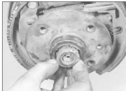
10.6a Fit the outer bearing race . . .
