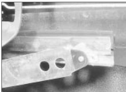
18.6 Scissors lifting mechanism slider
