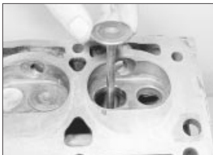
9.15 Fitting a valve to its guide
