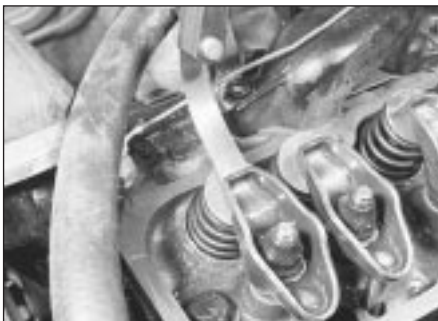
7.10 Checking a valve clearance
