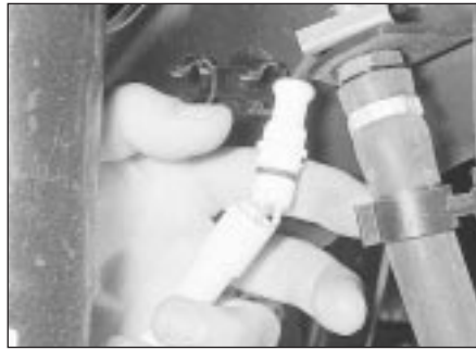
22.3b Separating a front sensor connector
