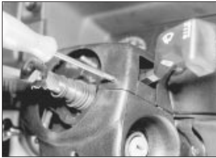
20.3a Removing an upper shroud securing screw
