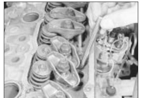
8.17 Removing the pushrods
