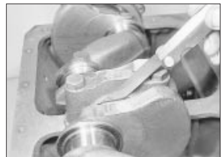
20.18 Checking the crankshaft endfloat
