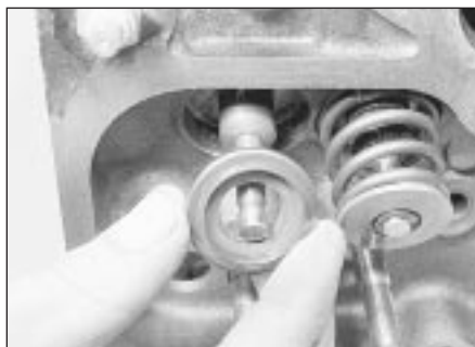
9.17 Fitting an exhaust valve rotator
