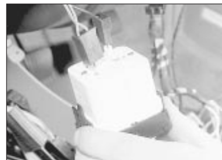
6.2 Removing the clock
