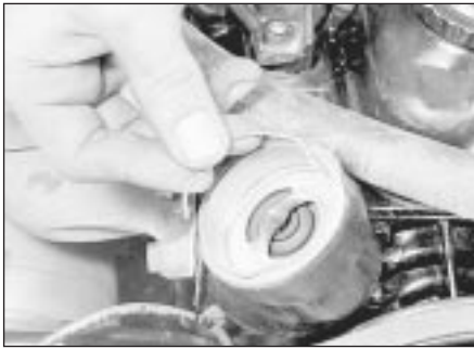
4.3a Remove the thermostat retaining snap-ring . . .
