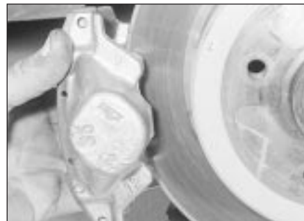
11.5 Removing the rear caliper
