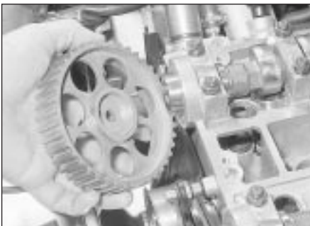
10.3b Removing a camshaft sprocket
