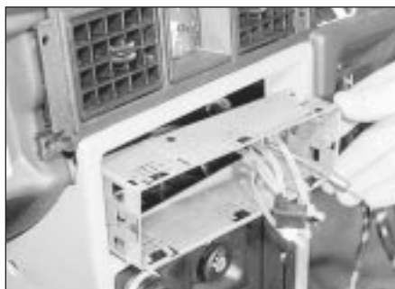
25.4 Removing the radio surround
