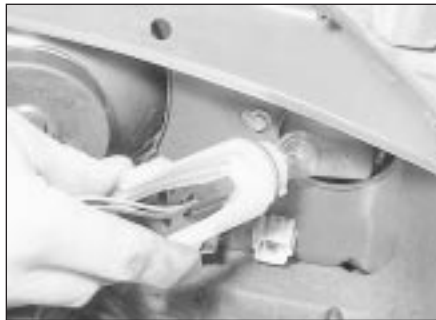
11.9 Removing a direction indicator bulb and holder
