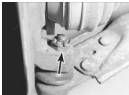
5.3 Control arm balljoint nut (arrowed)
