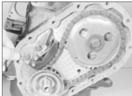
14.20 Fitting a new timing cover gasket
