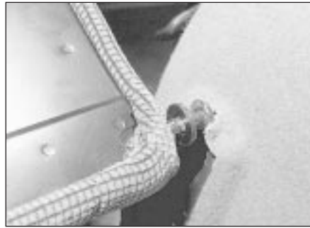
33.3b Seat pivot lifts out of hinge
