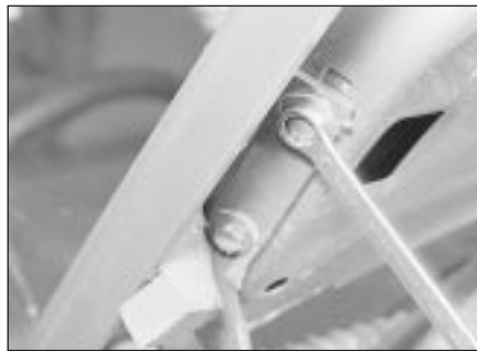
6.3 Removing a bonnet hinge bolt
