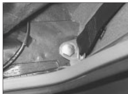
37.7c Rear seat belt floorpan mounting
