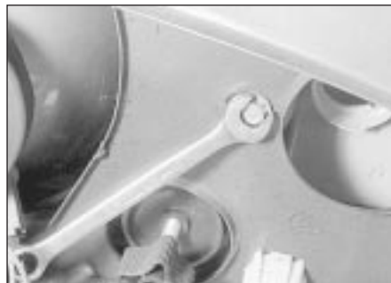
12.2a Undoing a direction indicator lens screw
